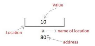
We can access the value 10 by either using the variable name **a** or the address 80F. Since the memory addresses are simply numbers they can be assigned to some other variable. The variable that holds memory address are called **pointer variables**. A **pointer** variable is therefore nothing but a variable that contains an address, which is a location of another variable. Value of **pointer variable** will be stored in another memory location.
