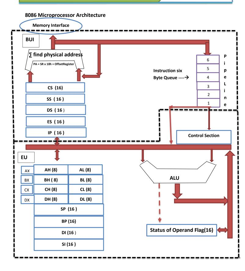
As a programmer of 8086, we must be familiar with the various register in the BIU bus interface unit and EU execution unit
